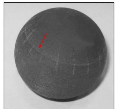
Figure 3: Model with a “seam” where the print job was interrupted.
