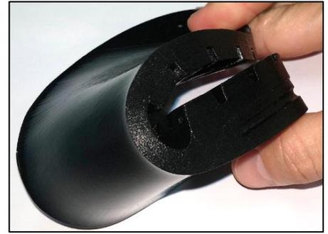
Figure 8: Painted prototype of a shoe sole
